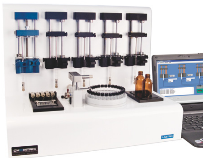
Figure 2. Illustration of the micro reactor development equipment, Labtrix® S1, supplied by Chemtrix BV.
