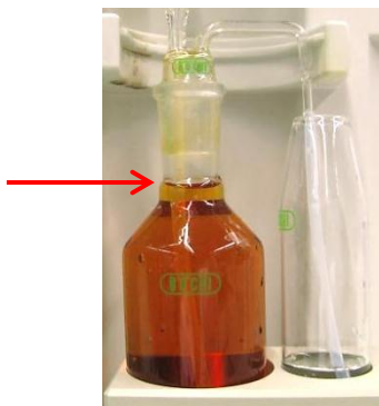
Figure 3: Distillation is stopped when the level of the distillate reaches the neck of the bottle.
