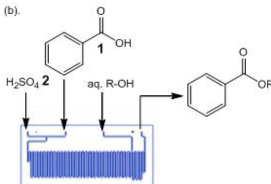
**Figure 1.** Illustration of (a). Labtrix® S1 the micro reactor development equipment used in this investigation and (b). a schematic of micro reactor (3023) set-up employed.
