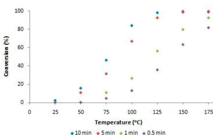
Figure 2. Summary of the results obtained for the continuous flow synthesis of methyl benzoate **3**.
