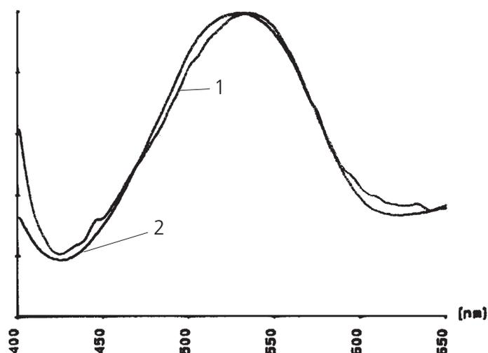
Fig. 2 VIS-spectra of hydrochlorothiazide standard (2) and urine sample (1)
