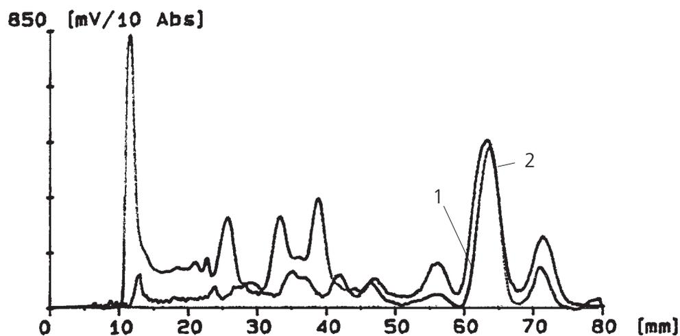
Fig. 3 Densitogram at 270 nm (1) and at 540 nm after derivatization (2). Hydrochlorothiazide, which was identified by UV- spectra, has reacted to an azo dye by derivatization.
