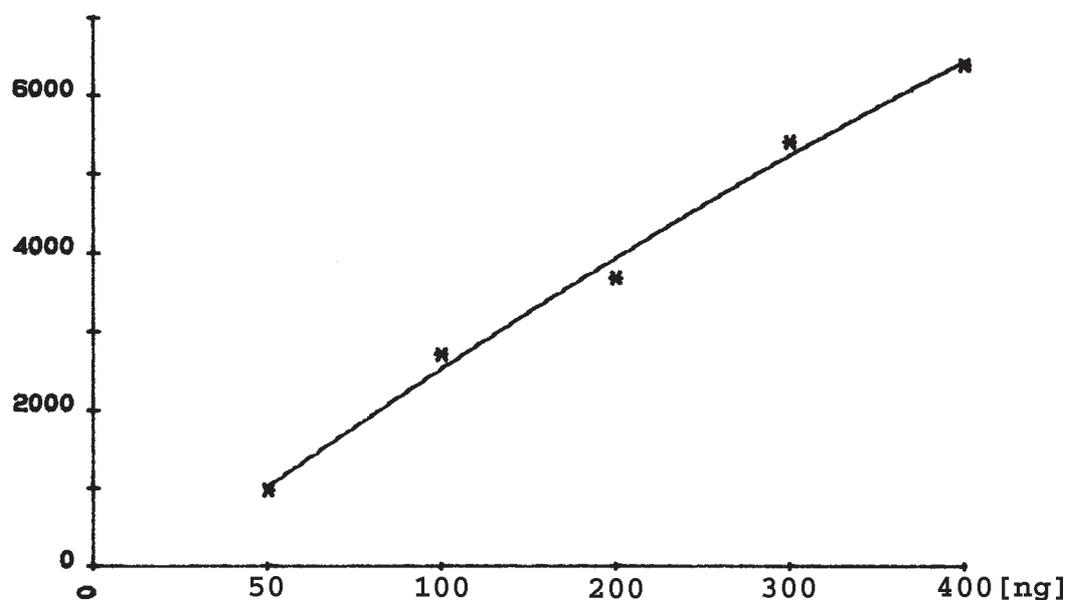
Fig. 4 Calibration curve for hydrochlorothiazide (absorbance at 270 nm): Evaluation via peak height with 2. degree polynomial. Calibration range 100-800 ng, corresponding to 0.2-1.6 mg/L.
