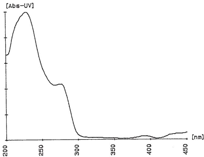
Fig.1 In-situ absorption spectrum of chlortalidone (Hygroton).
