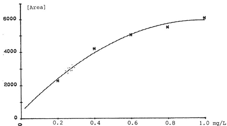
Fig. 3 Calibration curve of Hygroton in the range of 0.2-1.0 mg/L by second degree polynomial.
