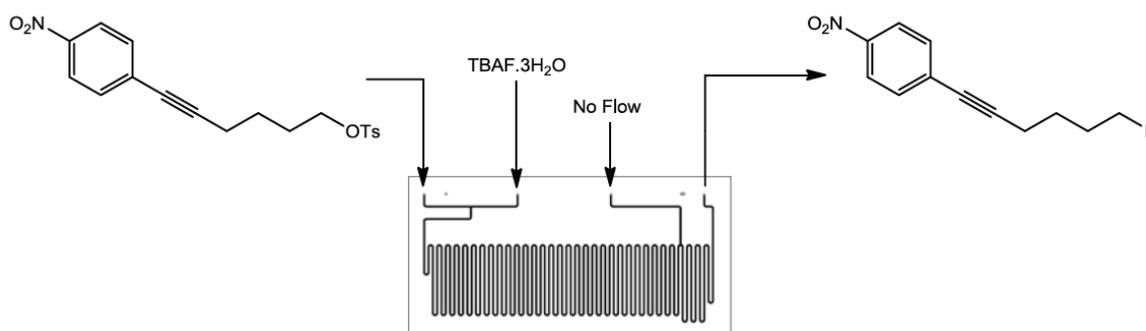
**Figure 2.** Schematic illustrating the Labtrix® reaction manifold used for the assessment of nucleophilic fluorination under flow conditions.
