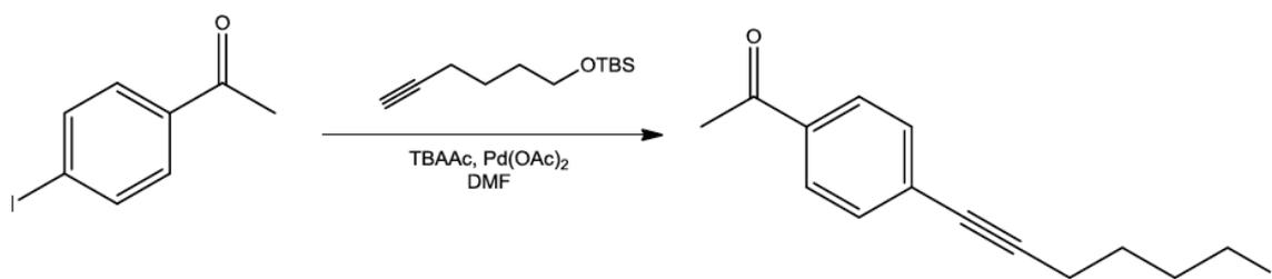
**Scheme 1.** Illustration of the model reaction used to optimise the Pd-catalysed coupling reaction.
