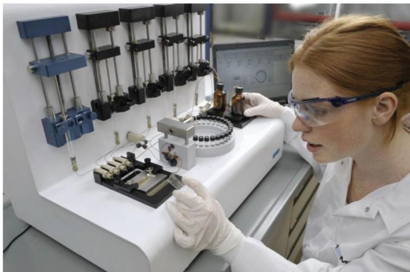
**Figure 1.** Illustration of Labtrix®-S1, the automated micro reaction development apparatus developed by Chemtrix.
