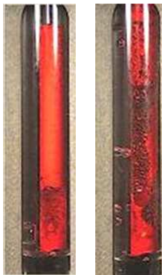
Figure 4. Influence of the immersion depth. Left: the upper edge of the sample was 10 mm lower than the water level. Right: the upper edge of the sample was 30 mm below the water level. On the right the sample rose out of the recording area.
