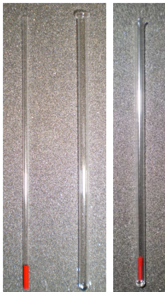
Figure 2. The lipstick sample outside (left) and inside (right) of the boiling point capillary.
