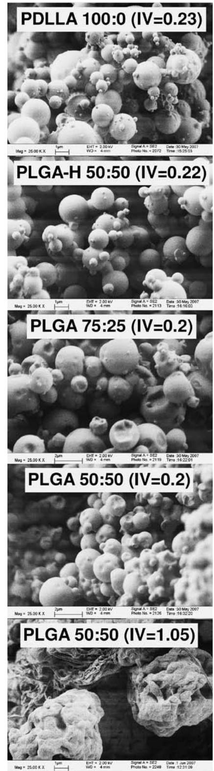
**Fig. 2:** SEM micrographs of spray-dried microspheres of different polymers.
