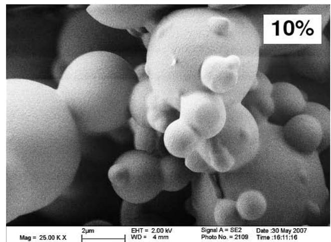
**Fig. 4:** SEM pictures showing PLGA (50:50) particles at different concentrations 1.5%, 5% and 10% (w/w).
