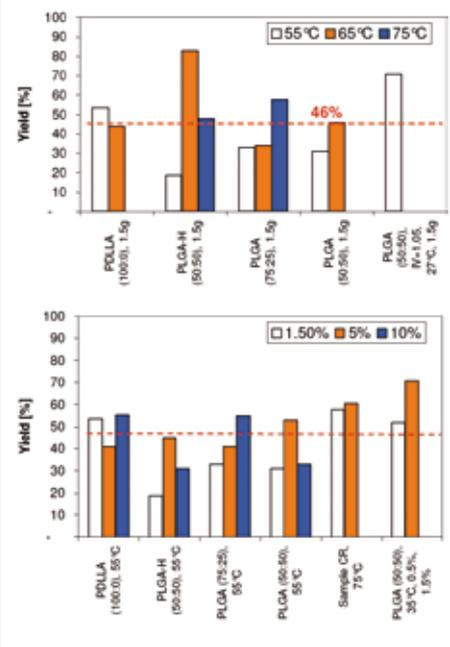
**Fig. 9:** Yield as a function of polymer type, temperature and polymer concentration.
