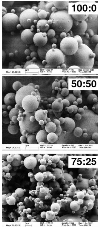
**Fig. 8:** SEM pictures of spray dried biopolymers with different lactide to glycolide ratio. PDLLA (100:0), PLGA (50:50) and PLGA (75:25).
