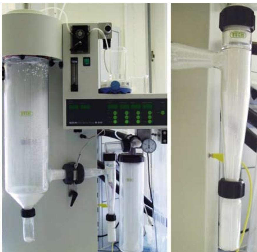
**Fig. 1:** Mini Spray Dryer B-290 with High Performance Cyclone during spray drying of bio-degradable polymers.
