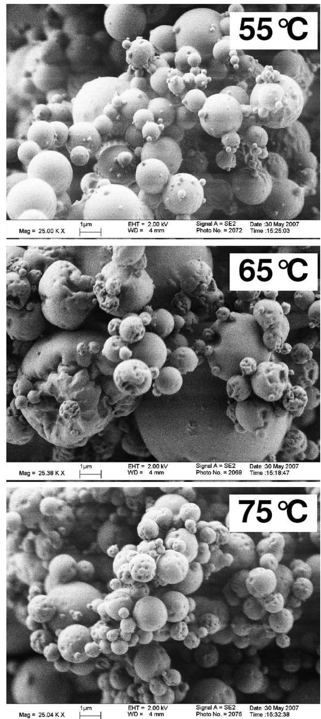
**Fig. 6:** SEM observation of the PDLLA spray dried powders obtained at 55°C, 65°C and 75°C inlet temperatures.
