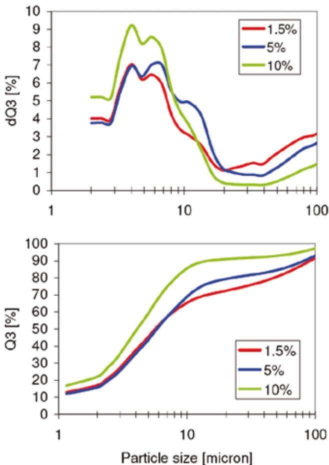
**Fig. 5:** Effect of different polymer concentrations (1.5%, 5% and 10%) for the PDLLA biopolymer on particle size.
