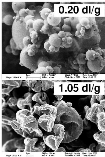
**Fig. 7:** SEM pictures of PLGA 50:50 polymers at two different molecular weights and inherent viscosities (0.2 and 1.05 dl/g).
