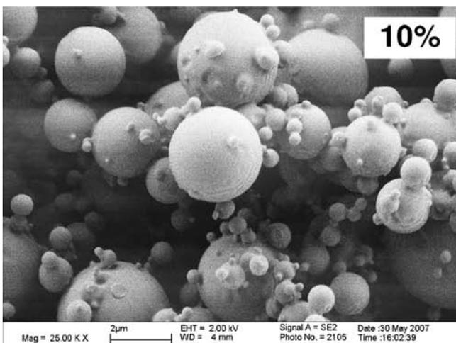
**Fig. 3:** SEM morphology of PDLLA microspheres prepared by spray drying at different polymer concentrations 1.5%, 5%, 10% (w/w).
