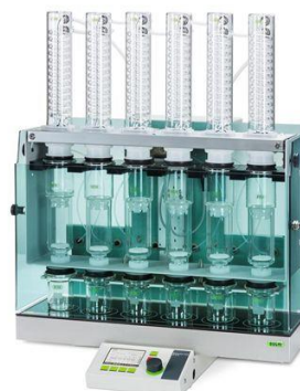
Figure 1: Extraction Unit E-816 ECE (Economic Continuous Extraction)
