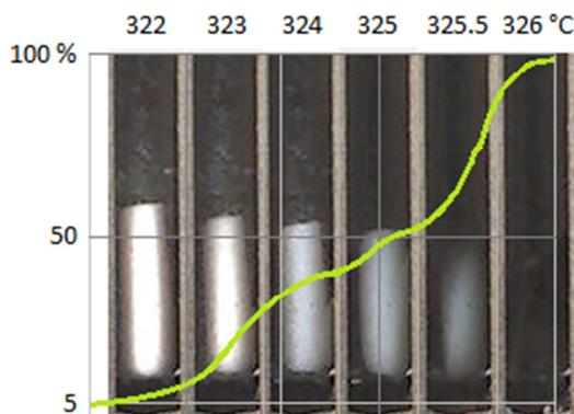
Figure 1. Temperature dependent melting process for PTFE. The green curve illustrates the corresponding melting grade recorded by the Melting Point Monitor 1.2 software. The melting range was observed between  $322.9 \pm 0.4$  °C and  $326.0 \pm 0.1$  °C.
