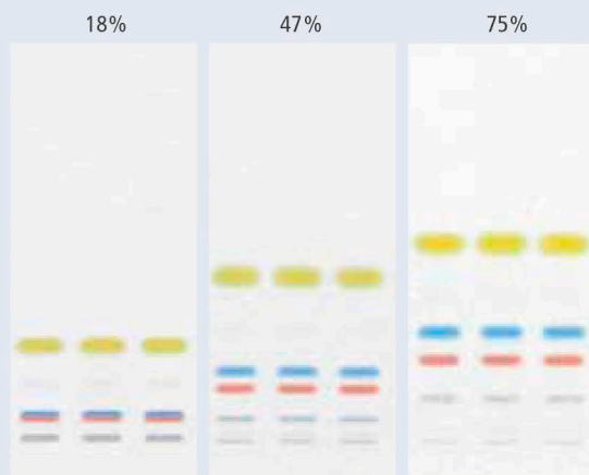
Influence of relative humidity ("activity of the layer") with the same solvent migration distance
