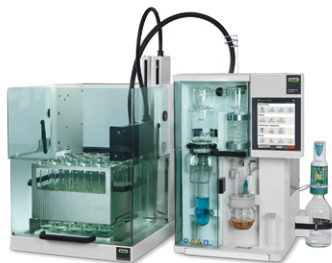
KjelMaster System K-375 / K-376 / K-377 Steam distillation, titration and auto sampling
