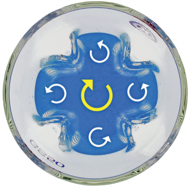
GS vessel principle (viewed from top)
