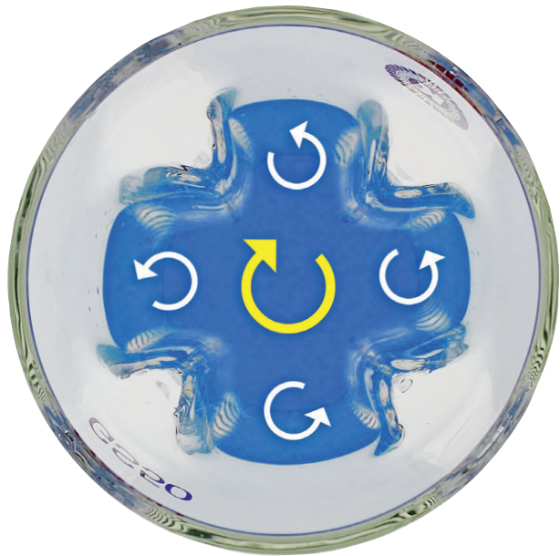
GS vessel principle (viewed from top)
