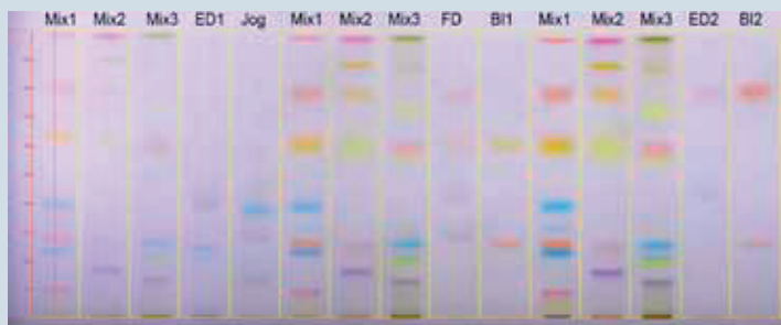
25 food dyes (split in 3 mixtures, application volumes of 1, 2, and 3 \mu\text{L} ) and 6 food samples (application volumes of 2 \mu\text{L} ; energy drink (ED), yoghurt (Jog), fruit drink (FD), bakery ink formulation (BI))
